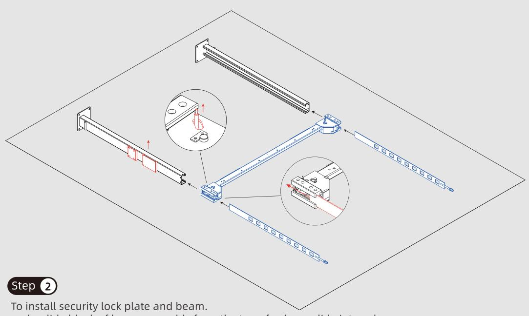
make slide block of beam assembly from the top of column slide into column. Pay attention to the direction of the column and beam.
