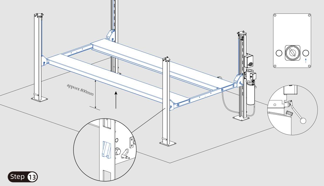
Press the up botton to raise the runway to the height of approx 800mm. Make sure all 4 locks well locked insde of ladders at the same height.
